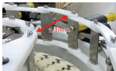
Accurate, repeatable adjustments to plus or minus 1mm.
